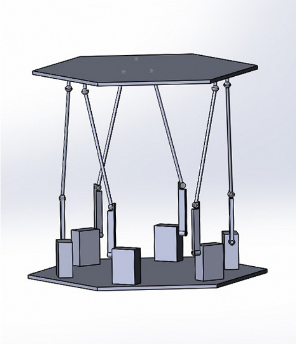
Fig. 1. 3D-model of the parallel manipulator with 6 rotary drives.
